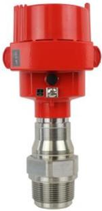
This threaded model of the BinMaster NCR-80 mounts simply through an existing 1-1/2" NPT opening. BinMaster's non-contact radar level sensor is a proven performer in powders and bulk solids, performing reliably in dense dust with accuracy within 0.2 inches. It can be precisely aimed to avoid the flow stream, internal structure, or sidewall buildup.
