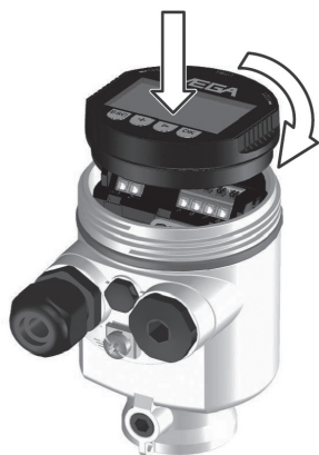
Fig. 6: Insertion of the display and adjustment module with single chamber housing
