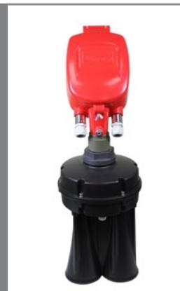
ket. Unlike the 26-GHz radar, radars using these high frequencies are reliable in dust. Their principle of operation is the same, but 80-GHz radar is less prone to erratic data or lost signals. High frequency radar has a 4° versus 10° beam angle for better precision and a 393-ft. measuring range.
