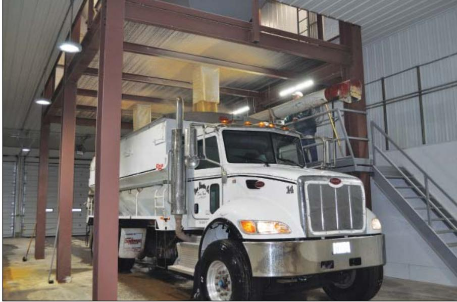
One of six feed trucks operated by Doon Elevator is loaded through one of two fixed spouts in the mill's single loadout bay. Trucks take an average of five minutes to load.
