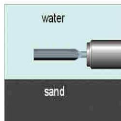
Function: A piezo system brings rod to vibrate at its resonant frequency. The vibrating system is tuned to work in water. If solid material covers the rod, it damps the vibration. An electronics circuit switches a binary output signal. When the rod gets uncovered, it starts vibrating again and the output switches back.
